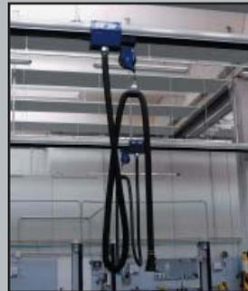
Sliding Suction Rail with Hose Drop & Balancer
